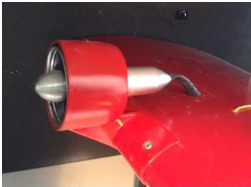
Pylon Mounted EDF
