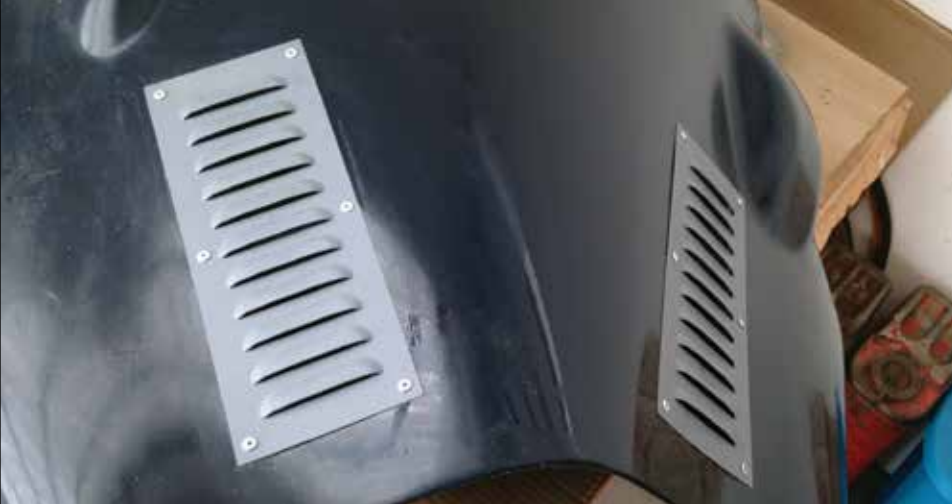
Small louvers on the bottom rear of the cowl helped draw air out.
