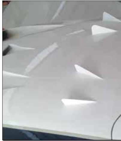
Left: Two small VGs, .43 inch tall, were tried first in front of each NACA duct. They helped, but not enough. The small VGs in the foreground were added later to help bring flow in when at a high angle of attack. Center and Right: Large VGs that are 2 inches tall and 5 inches long solved the problem. They are placed in pairs 15 inches in front of the start of each NACA scoop.
