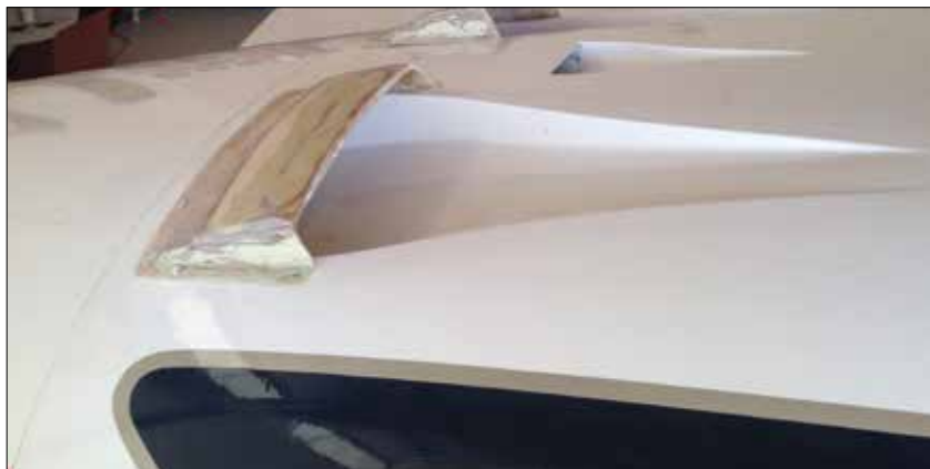
Small scoops protruded 1.5 inches above the fuselage surface. Large Scoops (not shown) were 3 inches high.
