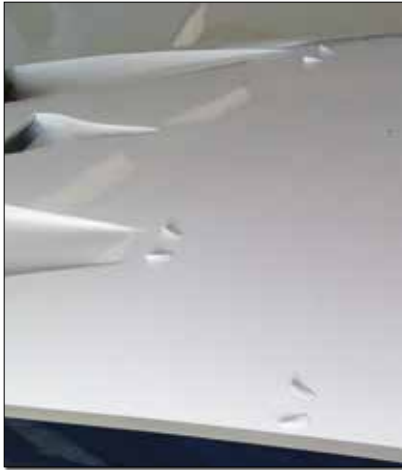
Left: Two small VGs, .43 inch tall, were tried first in front of each NACA duct. They helped, but not enough. The small VGs in the foreground were added later to help bring flow in when at a high angle of attack. Center and Right: Large VGs that are 2 inches tall and 5 inches long solved the problem. They are placed in pairs 15 inches in front of the start of each NACA scoop.
