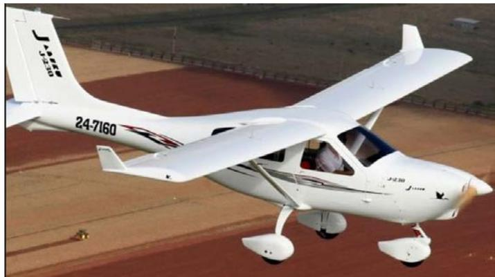
The J230 is ideal as it was originally designed as a four place aircraft and de-rated to a two-place to meet LSA rules. Thus, there is a large space aft of the seats and near the center of gravity for batteries and instrumentation. The EDF add-ons will be instrumented, as will the rest of the airplane, so that data can be taken on sets of EDF propulsors in full scale operation. Technology testing on this aircraft will begin in early 2018 and it will be renamed the “JabirWatt I”.
